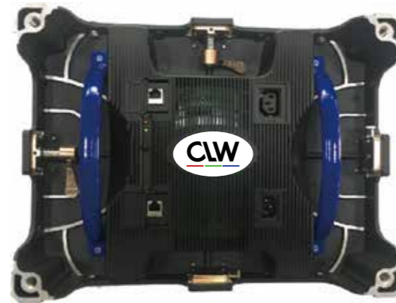
400*300 die-casting cabinet back side
